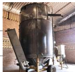
Figure 4: Warm air dryer – Loading end section
