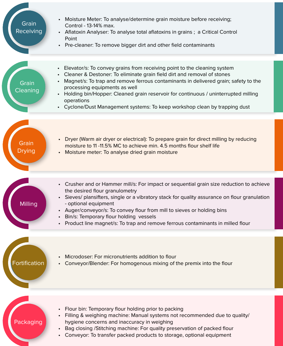
Figure 7: Process flow / equipment and their functions
