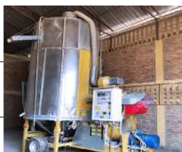
Figure 3: Warm air dryer – Burner end section
