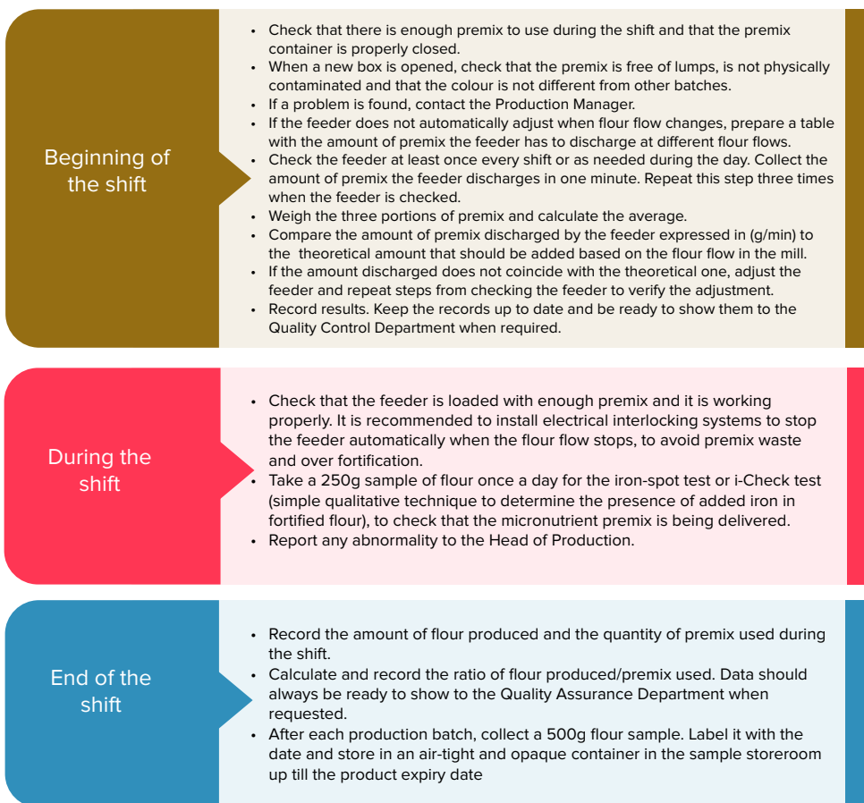
Figure 11: Maize flour fortification quality assurance procedure
